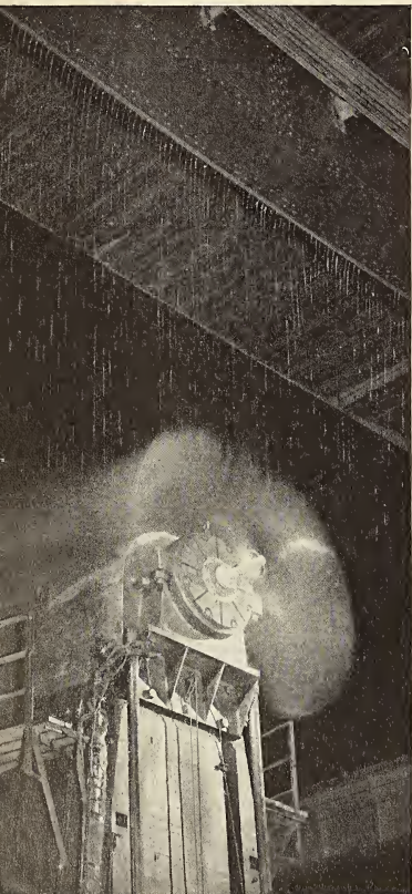
Made-to-order rain is used to test this prop's ability to hold up in rough weather.
